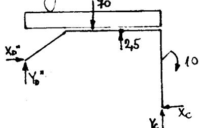
$$\left. \begin{array}{l} \sum M_C = 0 \\ \sum M_F = 0 \end{array} \right\} \Rightarrow \begin{array}{l} X_D = 13,043 \\ Y_D = 28,943 \end{array}$$
